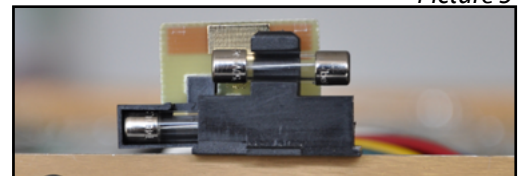
Picture 3 shows the fuse tray and the hidden spare fuse housing
